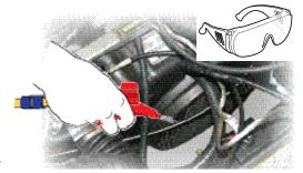
Regular maintenance of the cooling system is required to ensure an adequate supply of air to the cooling fins. Compressed air can be used for routine cooling system maintenance.
